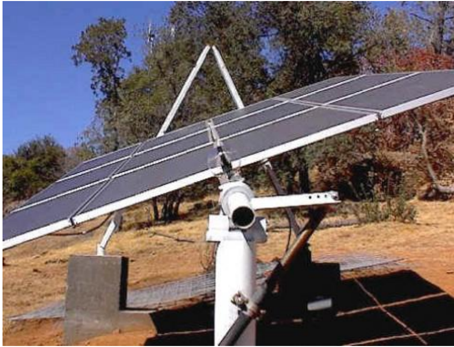
Fig. 1-7: The diagram of solar tracking system.
