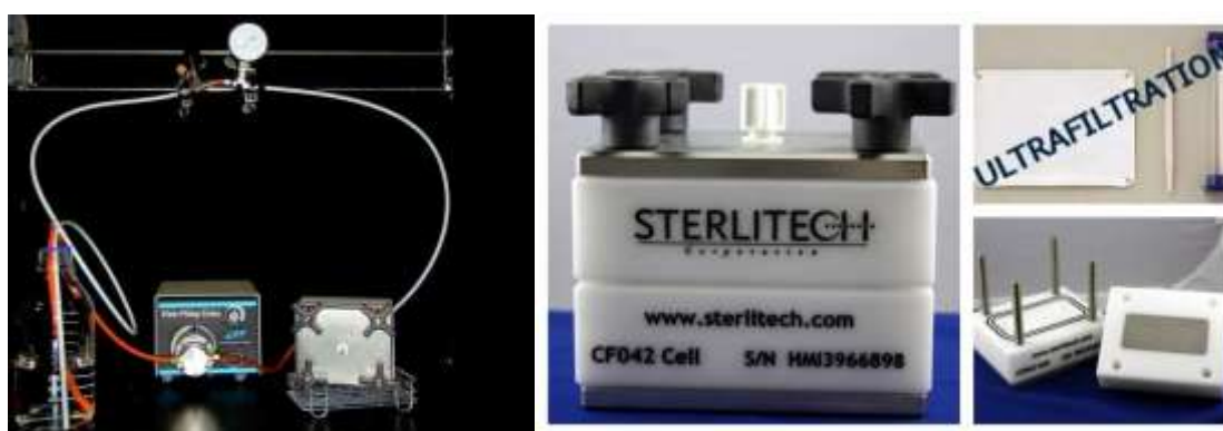
Fig 6. The schematics of a cross-flow filtration module and the filtration cell.
