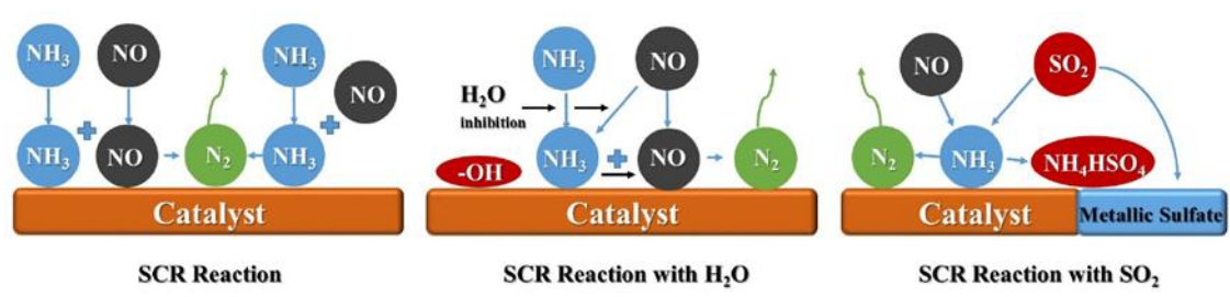
Figure 2-8. Effect of the H 2 O and SO 2 poisoning effect during SCR 53 .
