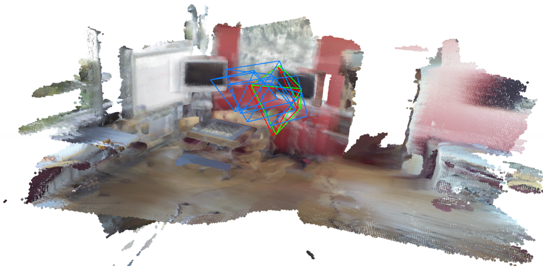
Fig. 1-1 Visualization of our localization procedure. The green one denotes the ground truth pose of query image, the blue ones denote the candidate image pose obtained by image retrieval, and the red one is the result pose estimated by our approach.
