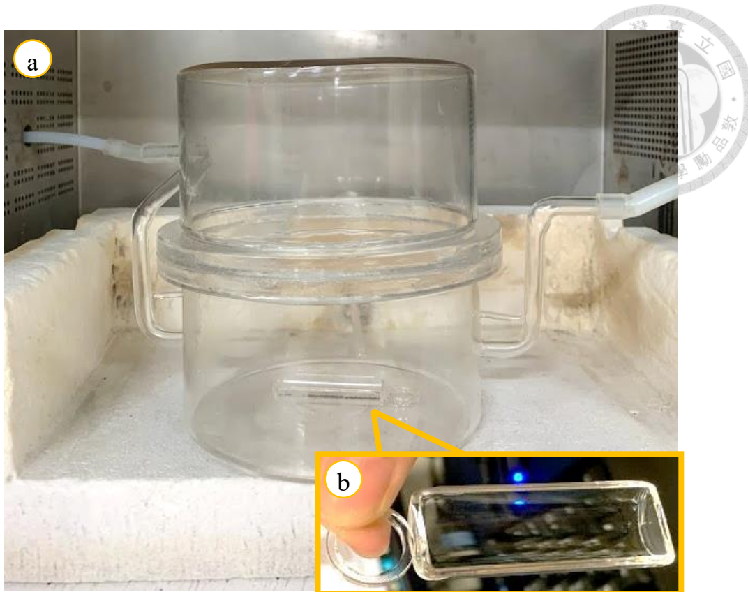
Figure 3-7 (a) the quartz reactor and (b) the quartz boat
