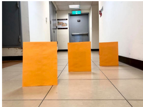
Fig. 4.6 Place cardboards at different distances on the floor, and use our LiDAR to scan its depth relationship.
