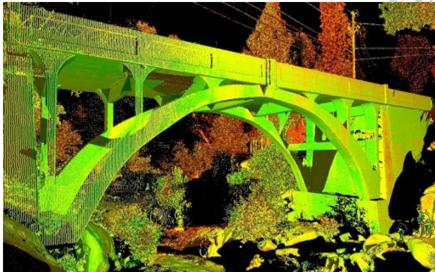
Fig. 1.6 Use Terrestrial LiDAR to scan the building and reconstruct the three-dimensional model of the building.[38]
