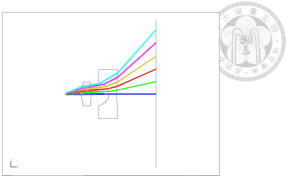
Fig. 3.9 The simulated 3D layout of the wide-angle lens, each line of different color represents the incident light at a different angle. The wide-angle lens system we designed is a combination of a positive lens and a negative lens, and the detailed structure of the lens surface is adjusted in different areas to improve the quality of the laser beam in each scanning area. The maximum beam angle of the wide-angle lens group is 104 degrees.
