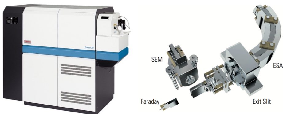
Figure 3.4 The high resolution inductively coupled plasma mass spectrometry (Thermo-Fisher Scientific™ ELEMENT XR) (a) Appearance (b) The detection system.
