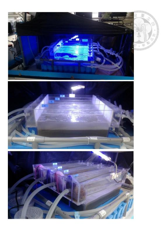
Figure S4-6. Photo diagrams for the start-up of the microcosm, including the pressure test (up), sediment incubation (middle; day -98) and rectifier added (down; day -97).
