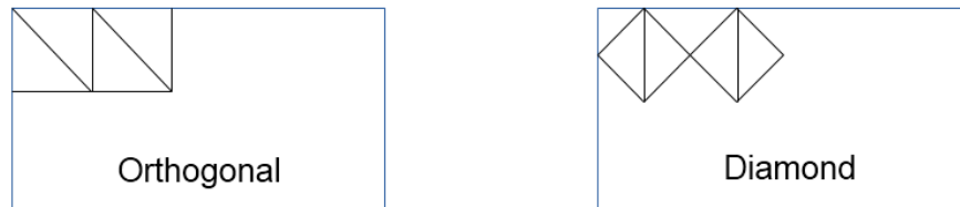
Figure 26 DMD orthogonal and diamond arrangements
