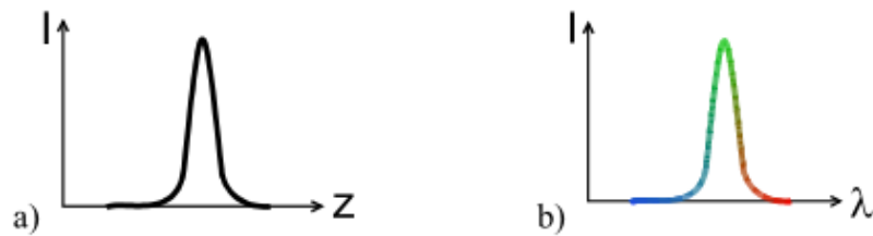
Figure 11 Confocal intensity signal a) with mechanical depth scanning and b) with chromatic depth scanning [9]
