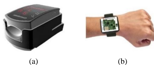
Fig. 1.4 PPG devices of (a) Pulse oximetry, and (b) Wrist-type PPG sensor watch [13]
