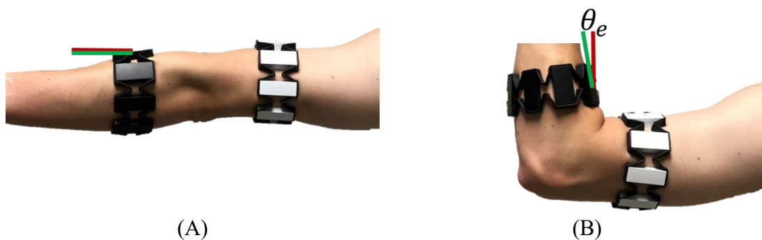
Fig. 3.4 Example of an inaccurate sensor measurement caused by muscle deformation.
