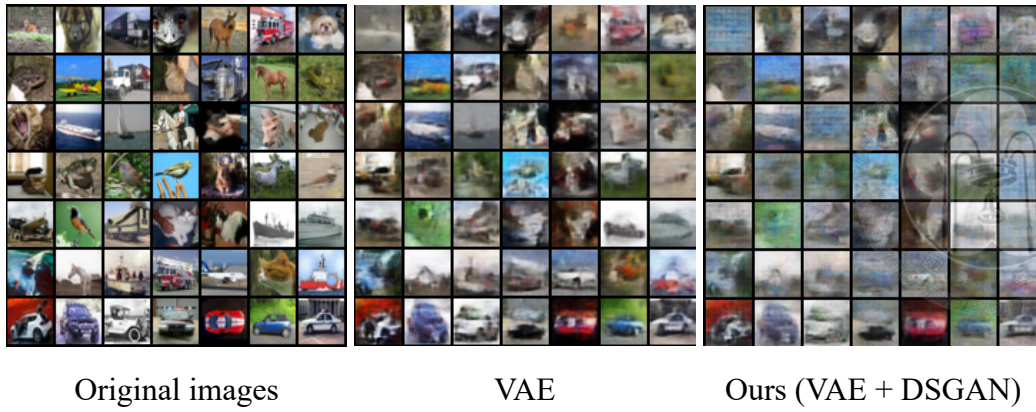
Figure 6.4: Comparison of the reconstructed results of VAE and our method. Seen class, which is at the bottom of the images, is car. Other rows are images from unseen classes. Our method exhibits a relatively larger gap, in terms of reconstruction error between seen data and unseen data, than VAE.
