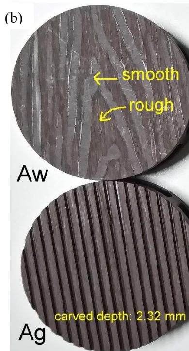
Fig. 11 (a) side view of specimen (b) wood grain pattern and grooved pattern (opposite sides) (c) group A with plain surface and perforation design.
