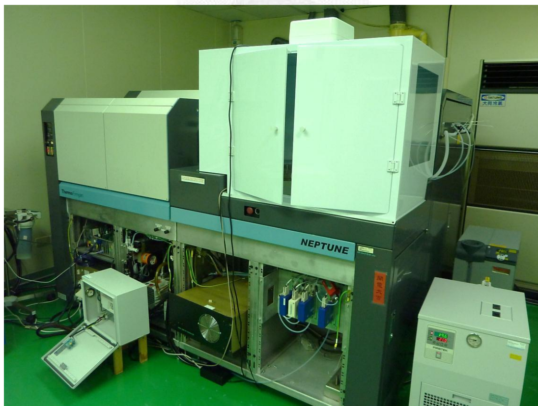
Figure 3.1 A MC-ICP-MS, Thermo Electron NEPTUNE, equipped with a class-100 PP hood on working bench.
