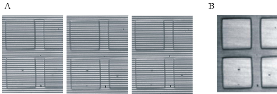
Figure 2-3. (A) Modulated images shifted by 1/3 periodic phase. (B) Reconstructed image with square-law detection principle. [18]
