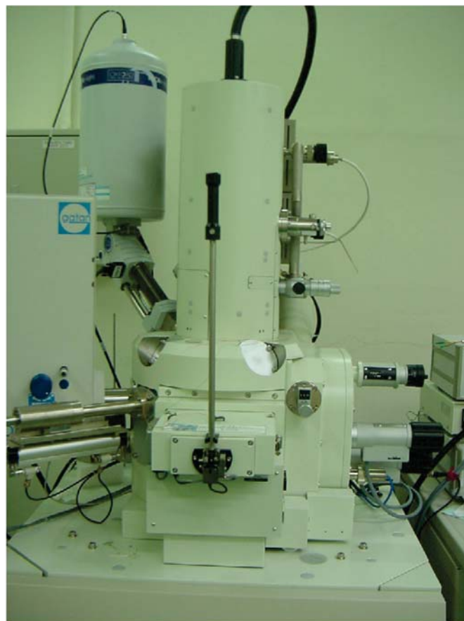
Fig. 3.3 Photo of scanning electron microscopy (JSM-6500F, JEOL)
