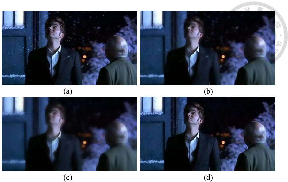
Fig. 5.21 Comparison of snow “streak” removal results: (a) the original snow image; the snow-removed version via: (b) Xu et al.’s method with the guided filter [4]; (c) Xu et al.’s method with the refined guidance image [4]; and (d) the proposed snow removal scheme.
