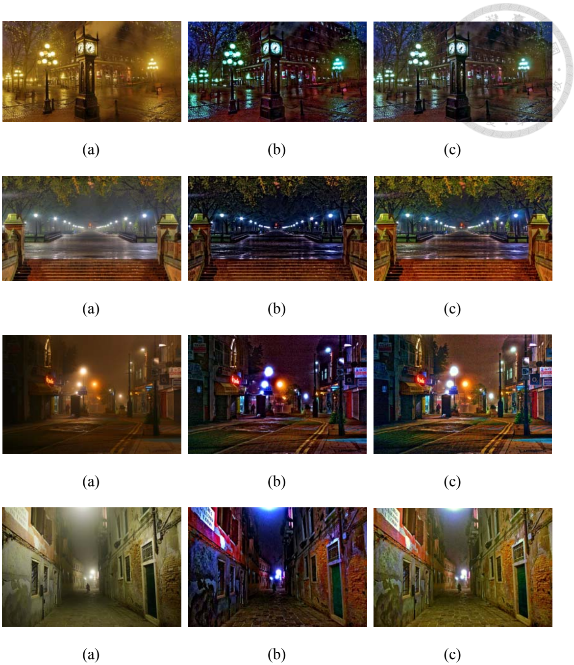
Fig. 3.18 Comparative results of the proposed method and the conventional methods on the nighttime haze images. (a) The input nighttime hazy images. The dehazed images obtained by (b) Pei et al.'s method [32], and (c) the proposed method.
