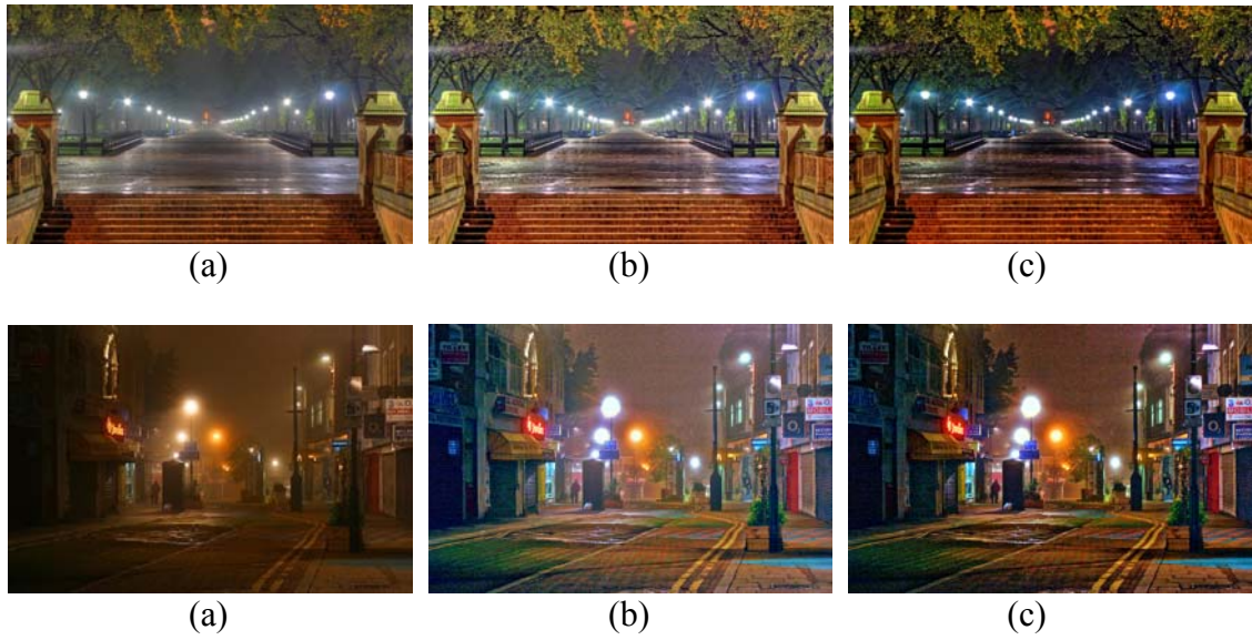
Fig. 3.11 Insufficient brightness and non-uniform distributed haze compare with BFLCC post-processing. (a) The input nighttime hazy image. (b) Final dehazing image. (c) Final dehazing image with BFLCC post-processing.
