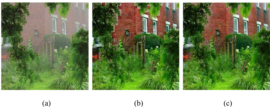
Fig. 3.4 Comparison of the dehazing result under two different cases of transmission map t . (a) Input hazy image. (b) Results for the block-based transmission map. (c) Results for the pixels-based transmission map.
