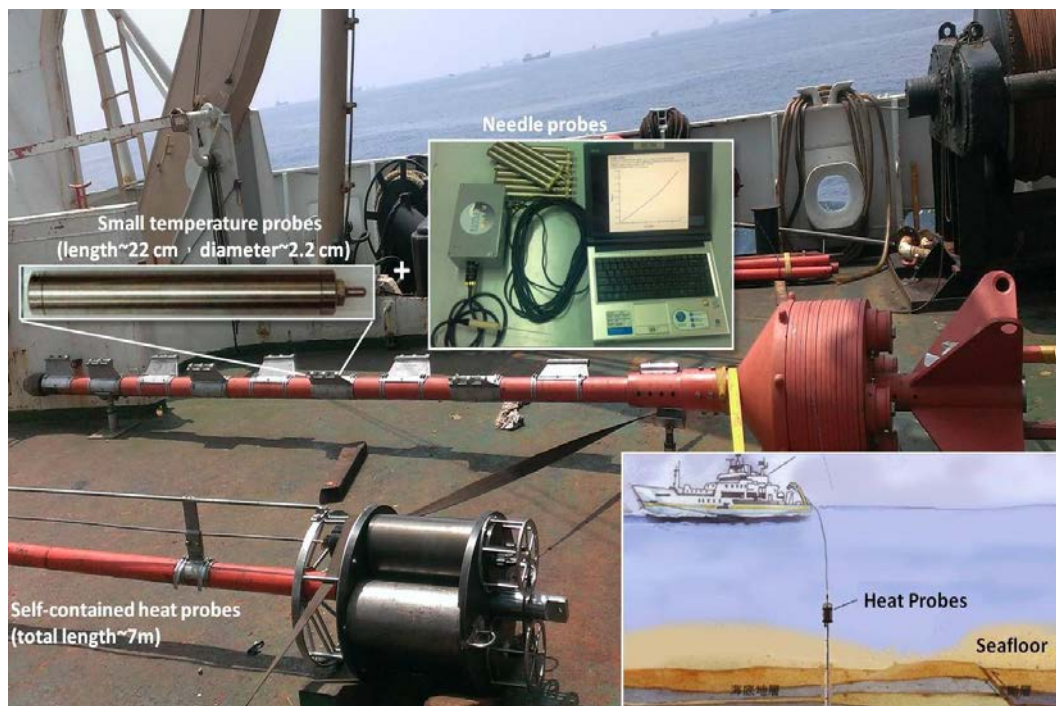
Figure 2-12 Two major types of ship-operated underwater instruments are used in marine geothermal investigations currently (which developed and improved by Prof. Shyu's Geothermal Lab, Institute of Oceanography, National Taiwan University): One is Lister-type heat probes (bottom), which is self-contained with multi penetration heat probes to measure both thermal gradients and conductivities of sediments in-situ; another type is small temperature probes which use miniature temperature loggers (MTL) attached to a solid-steel lance or a core barrel to measure thermal gradients (middle). If we use MTL, we have to use additional needle probes (center) to measure the thermal conductivities of the sediments.
