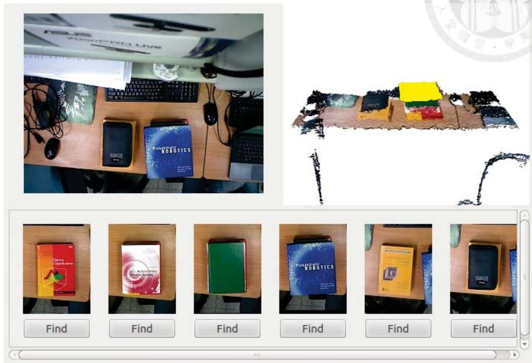
Figure 3.8. The interface of the desk object search system. A user can click the "Find" button with the photos at the bottom which corresponds to an object on the desk. The top left is the RGB image of current scene; while the top right is the visualizer that shows the 3D models in which the user's query object is indicated with yellow color.
