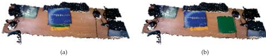
Figure 4.9. The result of experiment for taking out an object from the bottom of another object. (a) is the scene before moving, while the outcome after moving is showed in (b).
