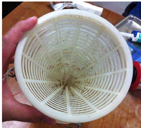
Fig 2.13. Top view of the fish trap. The hole in the middle is the entrance to the trap which has a diameter of 3cm.
