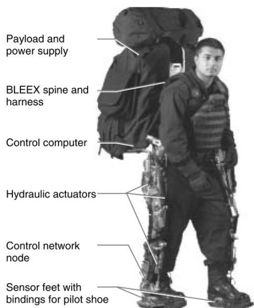
Figure 1.2 Berkeley Lower Extremity Exoskeleton (BLEEX)
