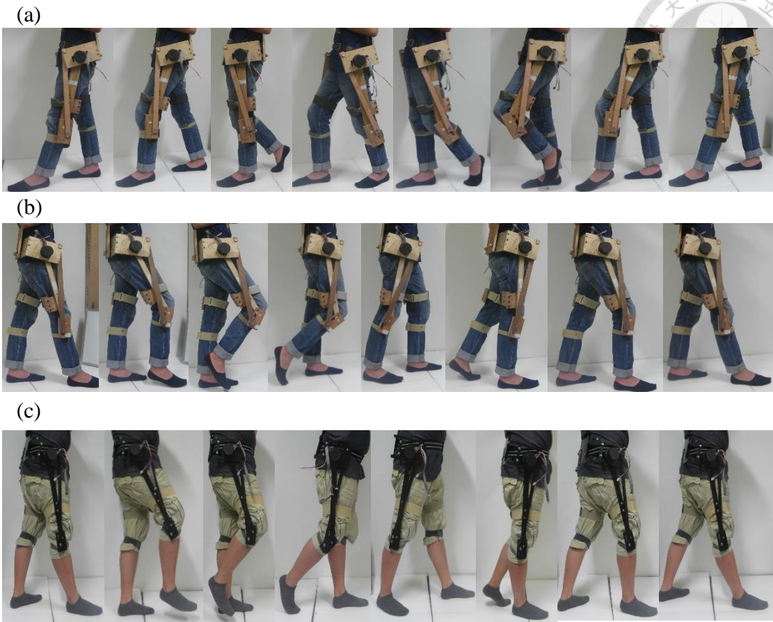
Figure 5.2 Result of wood and metal type with tester (a) A gait cycle with the tester wear the wood assist device on left leg. (b) A gait cycle with the tester wear the wood assist device on right leg. (c) A gait cycle with the tester wear the metal assist device on right leg.
