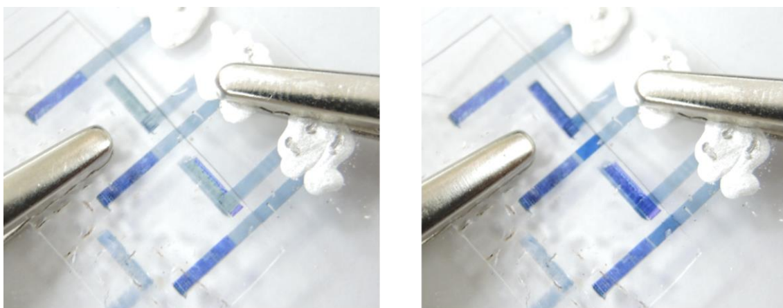
Figure 6.1 Seven segment display fabricated on PET with PEDOT and FeMEPE.
