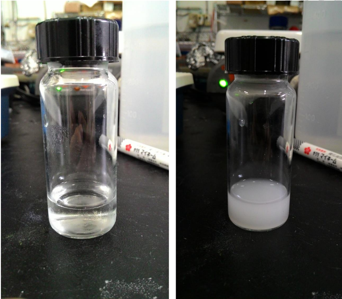
Figure 3-2 Color of solution below (left) and above (right) LCST
