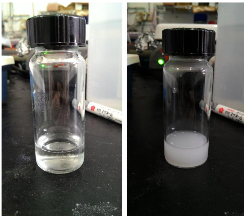
Figure 4-20 Color change of PPG-bis-adenine solution across LCST
