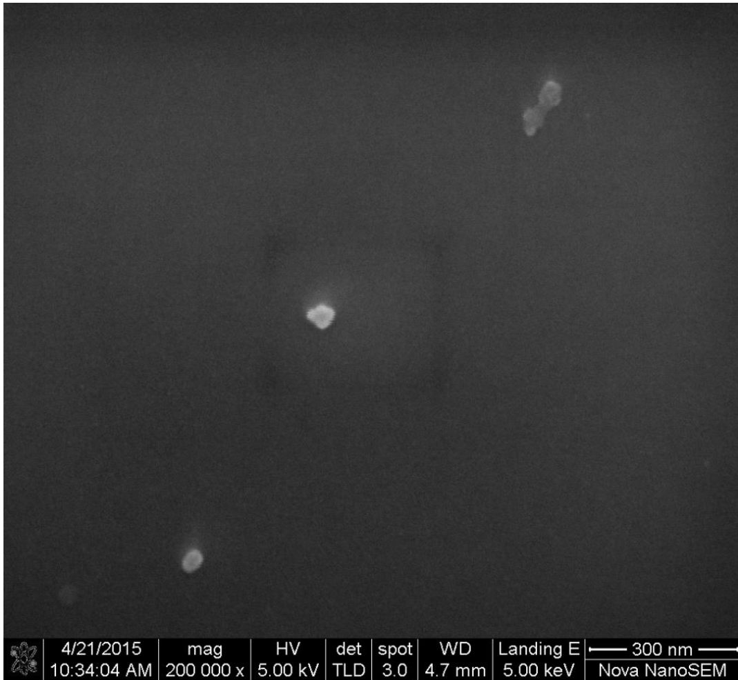
Figure 4-12 SEM image of nanoparticles of PPG-bis-adenine under 0.1 mg/mL
