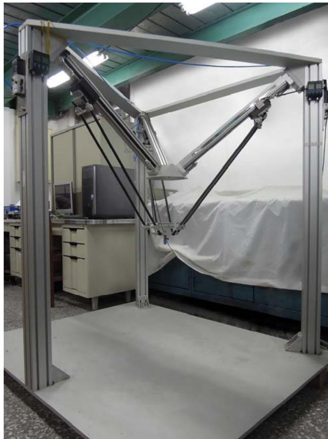
Fig. 2.3 Photograph of the three-axial pyramidal pneumatic parallel manipulator
