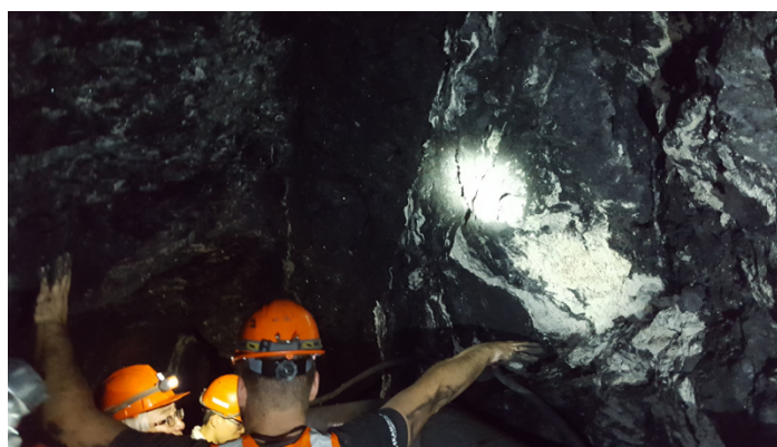
Figure 14 Sharp contact between shale and hydrothermally altered shale. The miners follow this contact in order to explore and exploit the emeralds.
