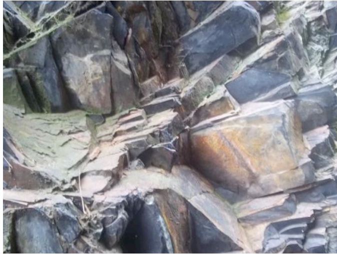
Figure 9 Joints with two predominant families in directions E-W / 45-50°S and N10-20°W / 85-90°SW.
