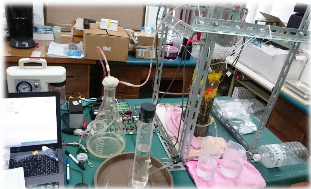
Fig. 4 Photo of calibration experiment construction used to test the accuracy of thermal dissipation methods-based sap flow.
