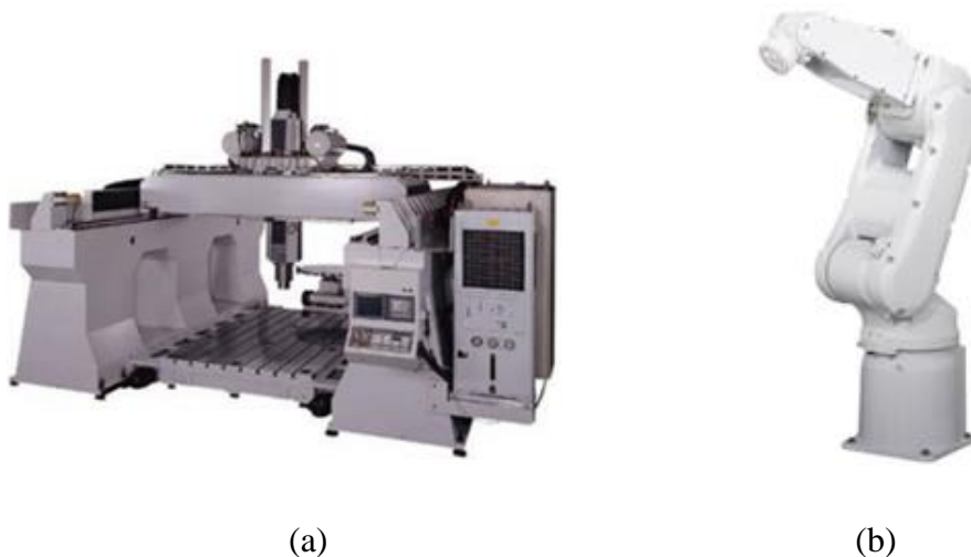
(a) (b) Fig. 2-2 Gantry-type machine and manipulator
