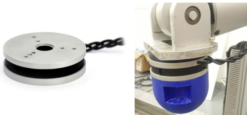
Fig. 2-6 The 6-axis F/T sensor is mounted on the wrist of each robot arm.
