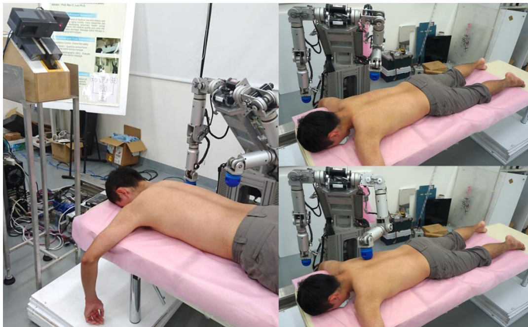
Fig. 5-15 Apply self-developed LRF to full body massage. Left: The LRF is mounted with a tilt angle in front of the massage bed. Upper Right: The LRF is scanning the subject's back. Lower Right: The dual arm robot executes pressing on subject's back.
