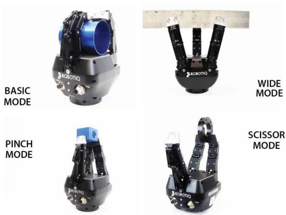
Fig. 4.9 Four operation modes of the gripper
