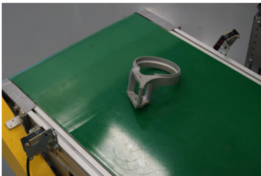
Fig. 2.2 The light sensor of the conveyor
