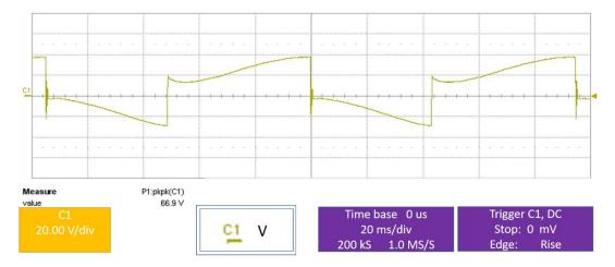
Figure 3-19 SCR malfunctioning waveform with overdriven voltage.
