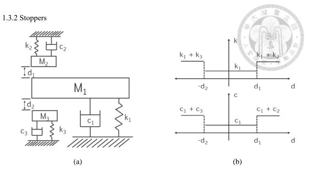
Figure 1-16 Model for stopper in forms of cantilever adopted from [26] (Redrawn) (a) MCK model (b) the stiffness k and damping c responding to the distance between the masses  $d_n$
