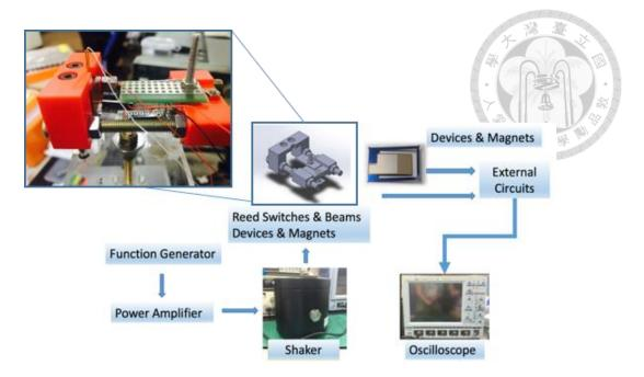
Figure 5-1 Experiment setup of the Micro PEH with reed switch SSH
