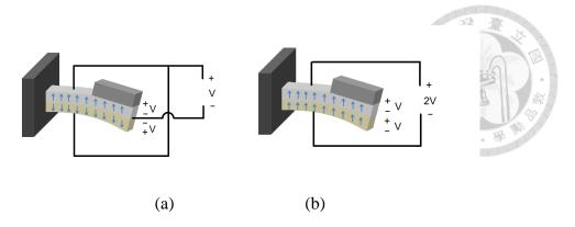
Figure 2-2 Schematic diagram of bimorph poling and connection (a) parallel connection (b) series connection
