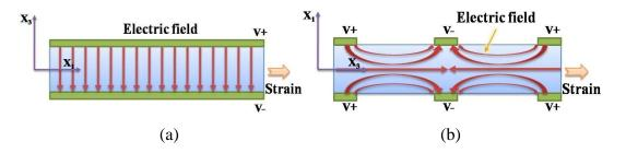
Figure 1-12 Working modes of the piezoelectric beam
