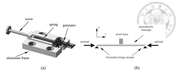
Figure 1-26 Tuning by preloading on axial direction (a) cantilever [53] (b) fixed beam [54]
