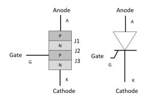
Figure 3-7 Schematic diagram of SCR
