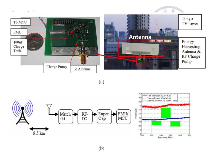
Figure 1-7 A radio frequency energy harvester, acquiring energy 6.5 km from the TV tower (a) Experiment Setup (b) The schematic of work flow (left) and the experiment results (right) [15]
