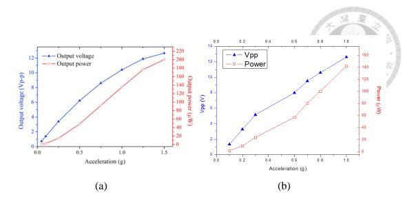
Figure 2-3 Power and voltage outputs of Micro PEH excited with varying acceleration levels (a) a typical uni-morph device (b) a typical bimorph device (in parallel),
