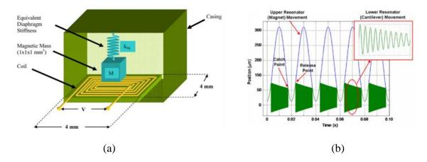
Figure 1-25 Up conversion design using electromagnetic energy harvesting [31] (a) Structure design (b) Trigger signal and up-converted signal
