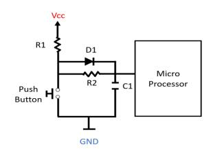
Figure 3-4 Conventional snubbers used in microprocessor controls
