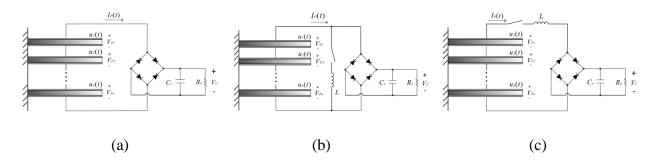
Figure 1-35 Circuit connection for cantilever arrays [83]
