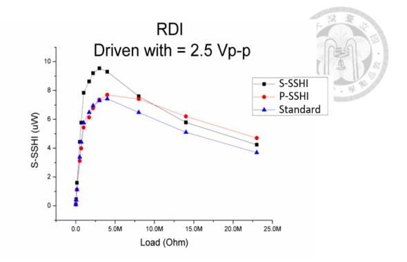
Figure 3-23 A low voltage driven experiment using RDI using piezoelectric voltage output was 2.5 V<sub>p-p</sub>
