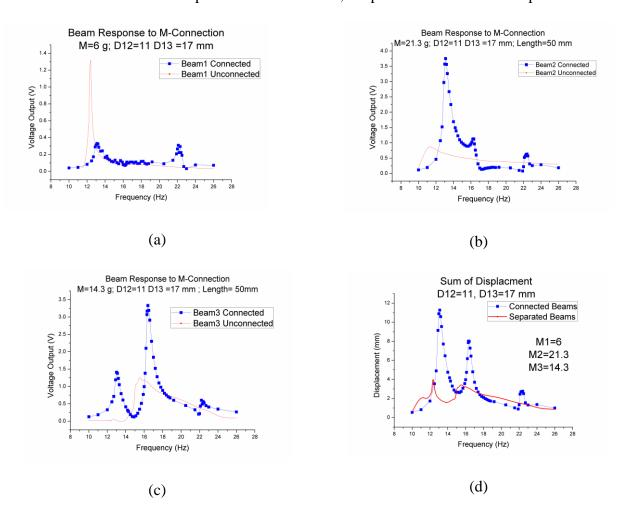
Figure 4-19 Experiment results of identical distances between beams. D<sub>12</sub>=11mm, D<sub>13</sub>=17mm.
