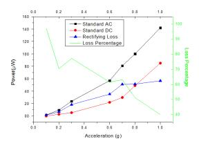
Figure 2-5 Rectify loss experiment of IC DB155
