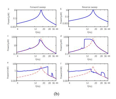
Figure 1-19 Output result of buckled-spring-mass systems
