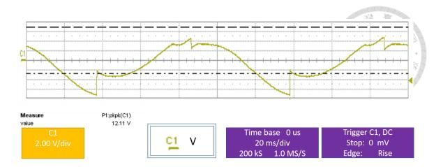
Figure 3-16 Piezo voltage output when high impedance is loaded at the RDI S-SSHI on  $3M\Omega$ , 0.07g, beam 1
