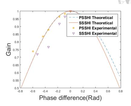
Figure 3-20 Phase difference relations to P-SSHI and S-SSHI gains. Externally powered switches used.
