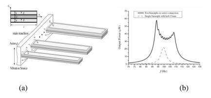
Figure 1-15 Cantilever array to create broad band [25]
