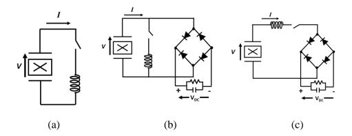
Figure 1-31 SSHI topologies with tagged voltage and current flow (a) Load Free Parallel SSHI (LF-P-SSHI), (b) Parallel SSHI (P-SSHI), (c) Series SSHI (S-SSHI)
