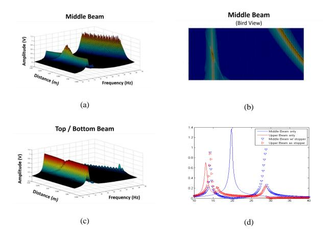
Figure 4-8 Simulation results for the symmetric 3-Beam alignment
