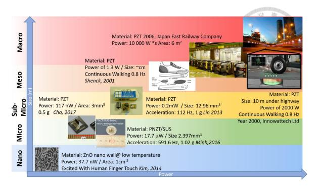
Figure 1-4 Energy harvesting devices in different scale in size corresponding to power output [7] [8] [9, 10]
