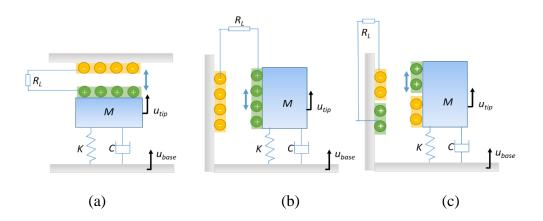
Figure 1-10 Three configurations of the electrostatic energy harvesting (a) gap changing (b) overlapping area change (c) counter electrode change
