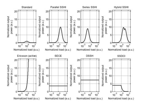
Figure 1-29 Normalized harvested powers under constant vibration magnitude. [21]
