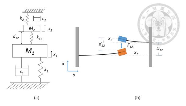
Figure 4-2 Magnetic interaction between two beams (a) Modeling by two MCK systems connected with a spring (b) Schematic diagram
