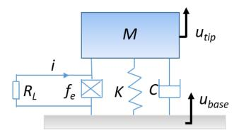
Figure 1-8 General spring mass damper model for transducers
