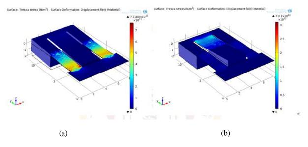
Figure 1-23 Stress simulation of a 2DOF beam [45] (a) on first resonance (b) on second resonance
