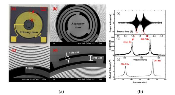
Figure 1-24 Spiral MEMS 2DOF device [46]. (a) Fabricated device (b) Experimental results
