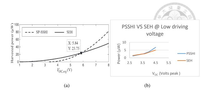
Figure 2-14 Comparison between the harvested power of self-powered SSHI and SEH (a) Theoretical results from [66] (b) Experimental result in this work
