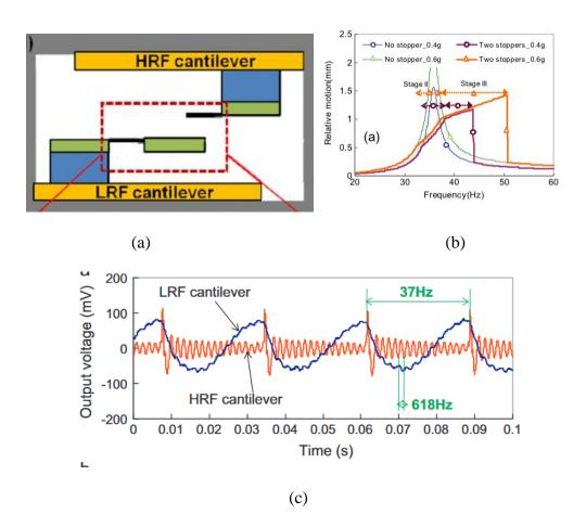
Figure 1-17 Results comparisons of different stopper distances on both sides (a) stopper on both side structure, with one side rigid and the other as an up conversion beam [30] (b) [26] (c) up converted result of [30]
