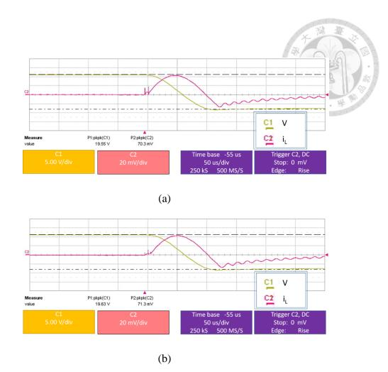
Figure 3-14 Current flow of filter snubbed LF-P-SSHI on switching (a) RDR (b) RDI 0.03g, beam 1
