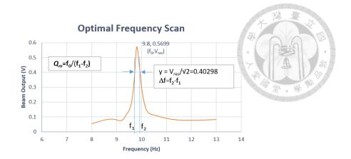
Figure 1-14 A typical voltage output respond to chirping frequency.
