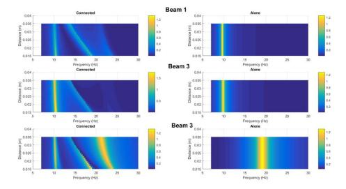
Figure 4-13 Bird view of frequency – distance –voltage for one fixed distance where  $m_1=21$ ,  $m_2=15$ ,  $m_3=4$ , g=0.1g showing the frequency shift when  $D_{13}$  is fixed,  $m_1$  placed 25 mm from the tip.
