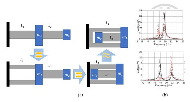
Figure 1-22 2DOF Structure design and results [44]
