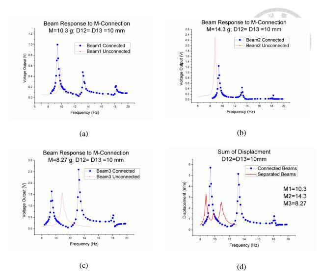
Figure 4-17 Experiment results of identical distances between beams. D<sub>12</sub>=D<sub>13</sub>=10mm.
