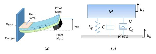
Figure 1-11 A piezoelectric cantilever based energy harvester (a) Schematic (b) MCK model
