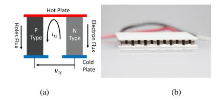
Figure 1-6 Thermal Energy Harvester
