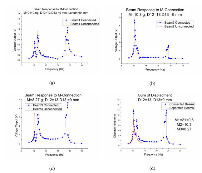
Figure 4-21 Experiment results of identical distances between beams. D<sub>12</sub>=13mm, D<sub>13</sub>=9mm.
