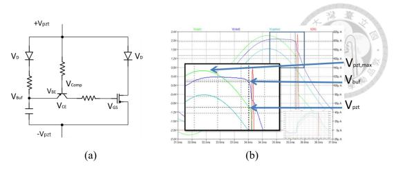
Figure 2-8 The voltage distribution on the smart switch
