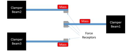
Figure 4-11 A new configuration for 3-beam alignments
