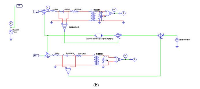
Figure 4-3 Implementation of the MCK model for simulation (a) block diagram (b) PSIM model
