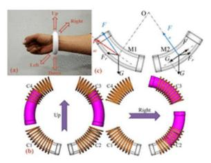
Figure 1-9 Magneto-electrical energy harvester wearable device with random movements[16] (Non-spring mass system)
