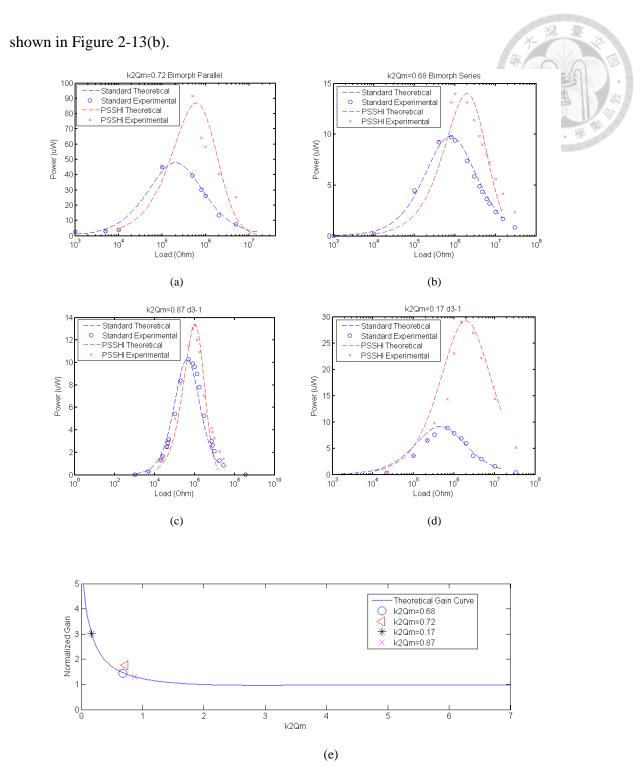
Figure 2-13 Experimental results of parallel SSHI with power sources enough to drive SSHI.(a) Bimorph in Parallel (b) Bimorph in Series (c) d<sub>31</sub>#1 (d) d<sub>31</sub>#2 (e) theoretical gain value Beam parameters can be found in Table 5.
