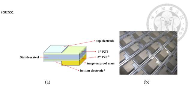
Figure 2-1 Schematic diagrams of the piezoelectric MEMS generator. [10] The starred content exists in the bimorph structure only (a) beam structure (b) fabricated beam.
