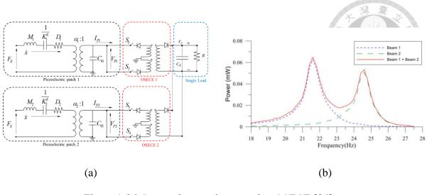
Figure 1-36 Connecting two beams using OSECE [84] (a) circuitry arrangement (b) experimental results
