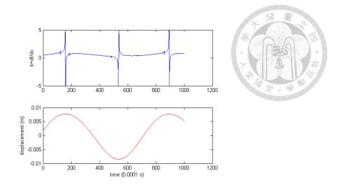
Figure 4-4 Simulation of the magnetic spring coefficient between beam 1 and 2,  $k_{12}$  corresponding to the changing distances between the magnets d<sub>12</sub>. Displacement on the lower refers to  $u_1$ , on resonance of beam 1
