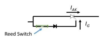
Figure 3-8 Unidirectional SCR de-bouncer
