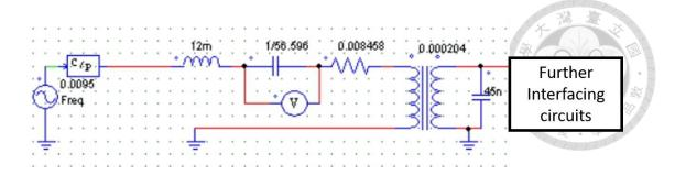
Figure 1-13 Equivalent circuit model of a single beam considering only the first resonance
