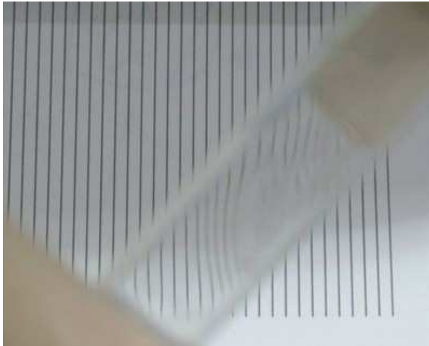
Figure 32. Poloxamer hydrogel bulk moving phenomenon in the centrifuge method.
