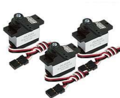
Fig. 2-8 DS410 Servo Motor [15]
