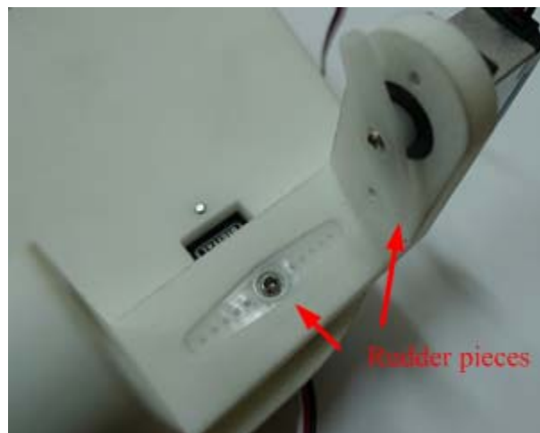
Fig. 2-3 The servo rudder piece used in the model
