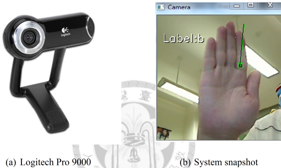
Figure 4.1: (a) Webcam (b) snapshot, the rectangle is center and the line denotes the posture direction
