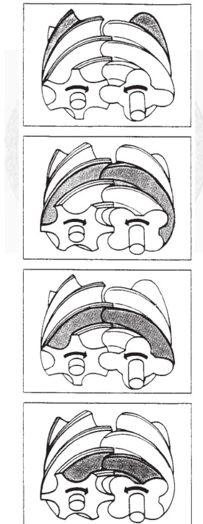
Figure 1-6 Operation process of a screw pump [3]
