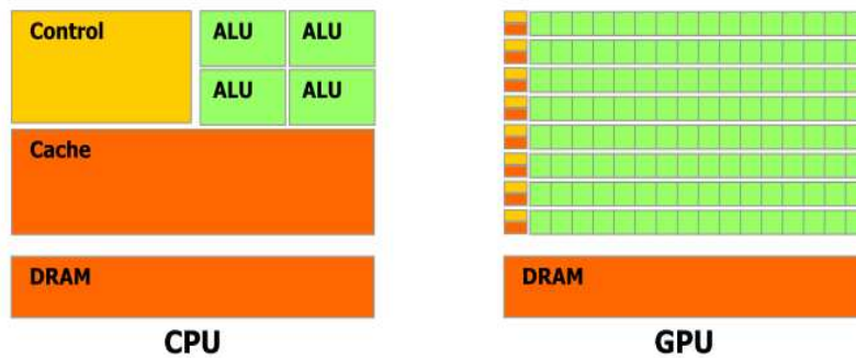
Figure 3.9 The GPU devotes more transistors to data processing. More precisely, the GPU is suitable for problems that are data-parallel. (CUDA Programming Guide Version 1.0. 2007)
