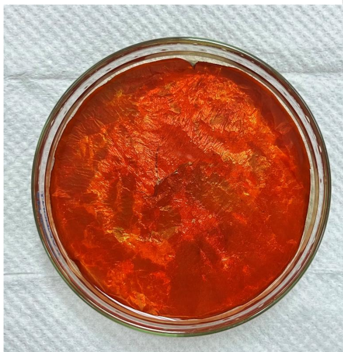
Figure 29 The photograph of COF Tp-PaSO 3 H.
