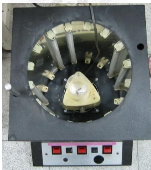
Fig. 3-2. Top-side view of photocatalytic batch reactor.
