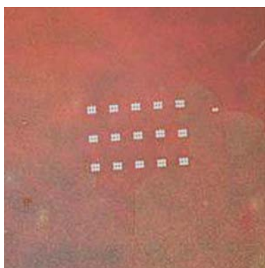
Figure 4.10: Optical micrograph of Ag/AAO template after patterning AAO and electrodepositing Ag.
