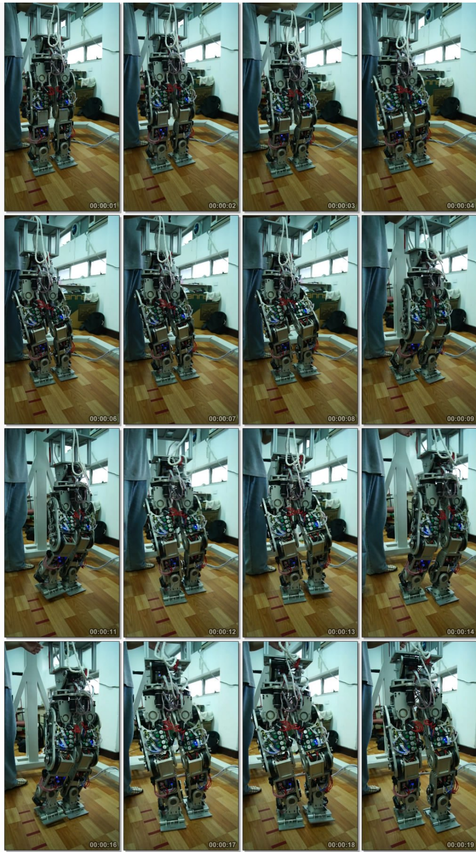
Figure 6-11 Humanoid robot, Voyager, walks with toe-off and heel-contact motions.
