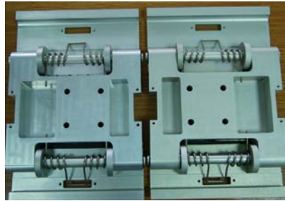
Figure 5-9 Mechanisms of foot pads with toe and heel joints
