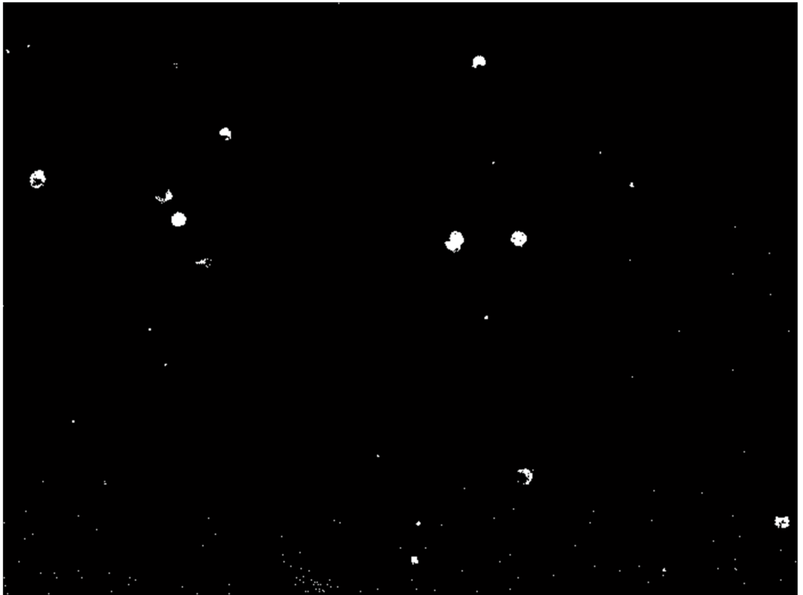
Figure 2-7 Threshold at third cluster, most of foreground elements are segmented with a small amount of noise, and some targets were segmented into many fragments. To remove noise and connect fragments of targets, we applied close operator first then open operator [8][9]. For convenient, the image was cut from origin one to display.
