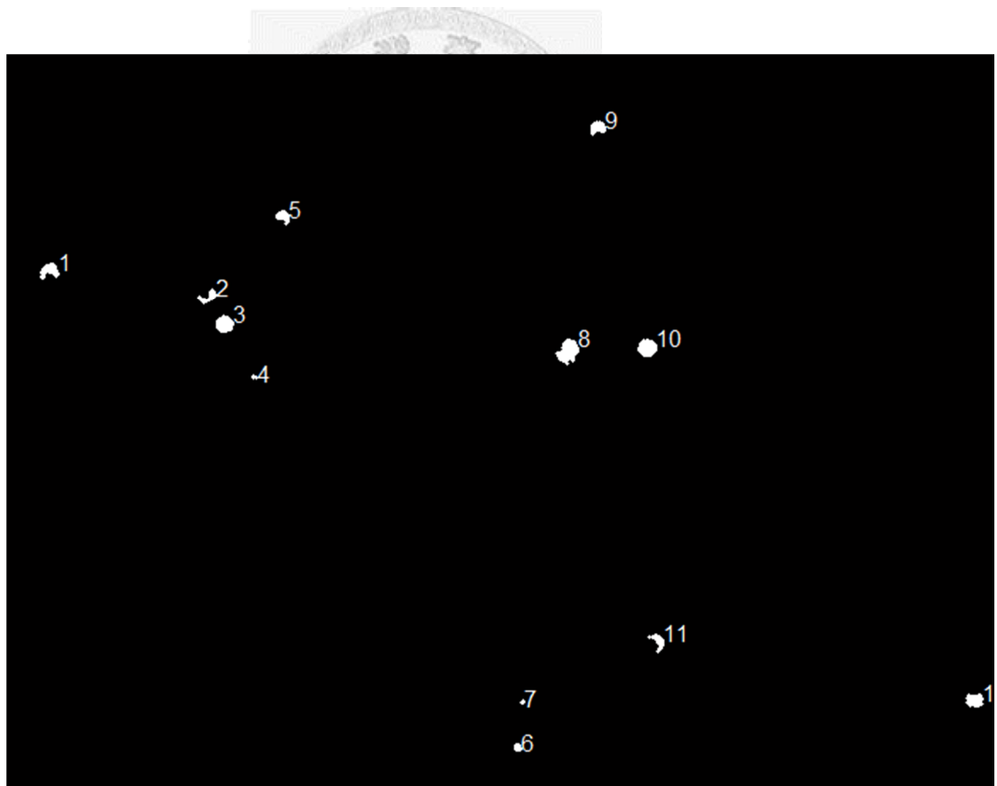
Figure 2-10 Target mask with label, the targets was applied area filter limit in 10 to 1000 pixels.
