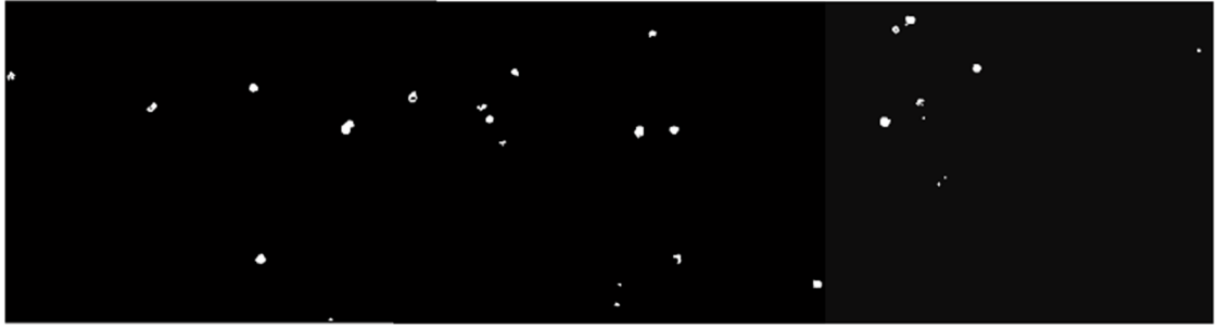
Figure 3-6 Result of union operation, the image mask merged according the position from scanner or computation, the repeated target were united.
