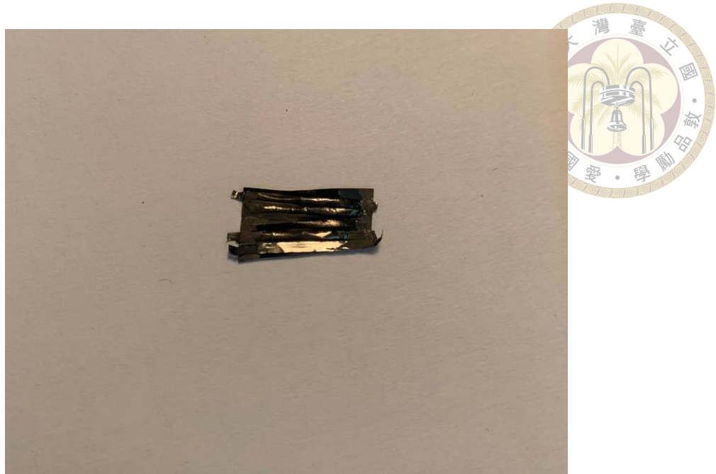
Figure 3.6: The aluminum foil stick across the Si substrate, so we can put AAO substrate between them.
