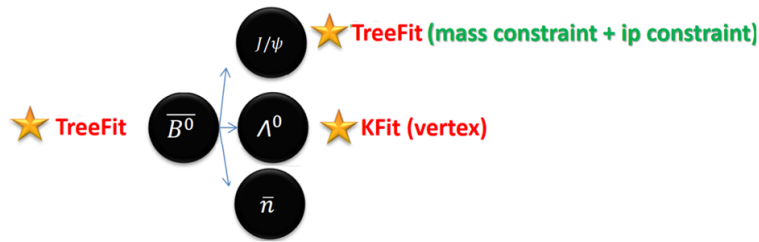
Figure 5.3: Vertex fitting strategy for the \overline{B}^0 \rightarrow J/\psi \Lambda^0 \bar{n} decay.
