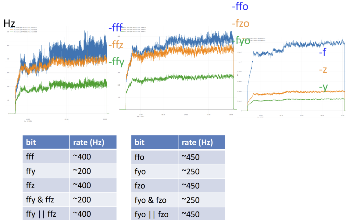
Figure 4.34: Trigger rates (Hz) of individual bits fff , ffy , ffz and ffo , fyo , fzo , together with their logical AND/OR combinations, during exp. 17 run #313. Following the geo-finder firmware update, ffz / fzo initially matched fff / ffo because GDL/GRL parameters were misconfigured, rendering the z_0 < 35 cm cut ineffective; after correcting the settings, the z -related rates decreased to the expected level, comparable to the y -related bits.
