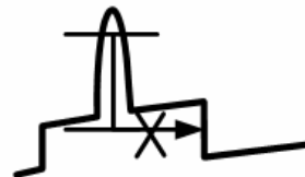
Fig. 3-11 The schematic detection of long-wavelength infrared at the \delta -doping layer. There may be SO level outside the \delta -doping well. The spectrum of the \delta -SiGe01 sample is only measured at the bias of 1 V. At 0 V, the photogenerated carriers cannot be collected.
