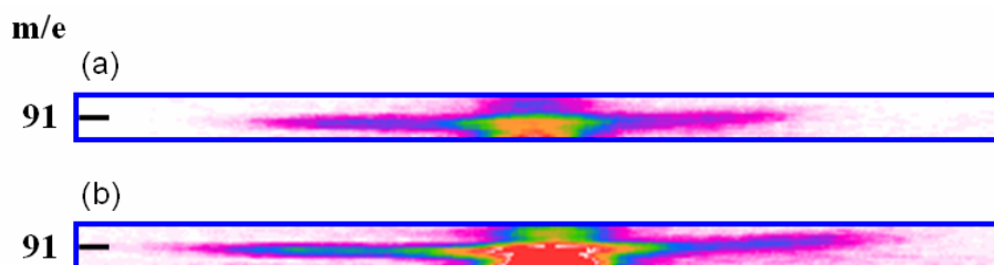
Figure 8. The ion image for m/e = 91 at (a) 12 \mu\text{s} and (b) 15 \mu\text{s} pump-probe delay time, respectively, with 248 nm laser excitation
