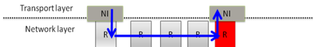
Fig. 2-7 Transport layer and network layer operation.
