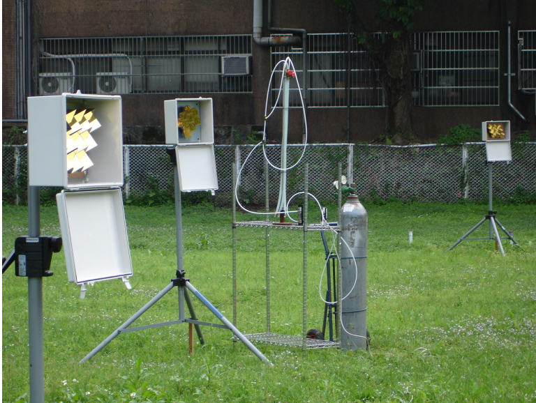
Figure 2.2 The tracer gas releasing device. The three vertical plastic tubes are at the same height of the retroreflectors.
