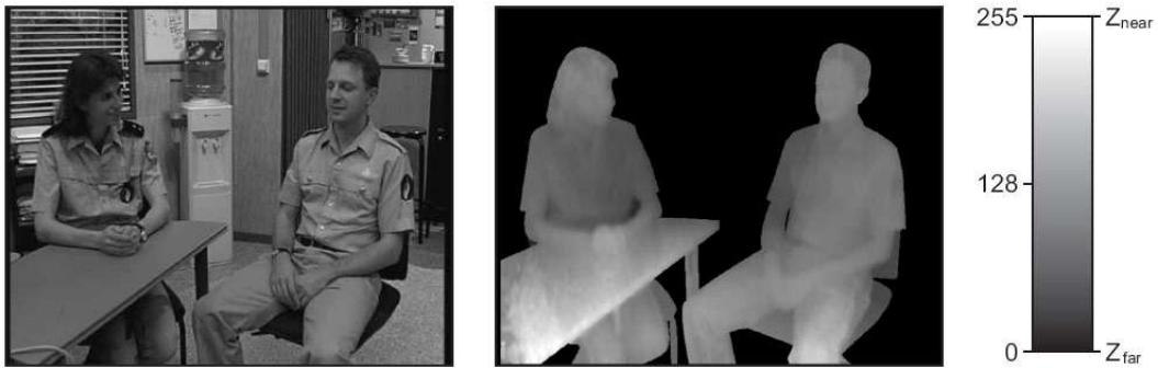
Figure 1.7: MPEG-C Part 3/ATTEST data representation format consisting of: 1) Regular 2D color video in digital TV format; 2) Accompanying 8-bit depth-images with the same spatial-temporal resolution [1].
