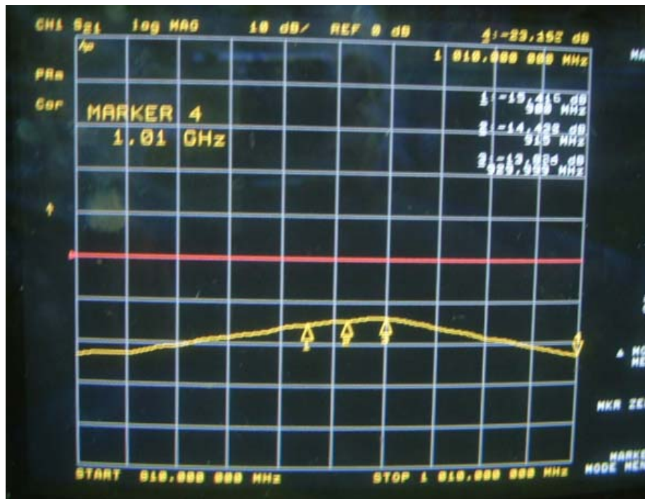
Fig. 4.23 Photograph of the curve of |S_{21}|^2 on the VNA.
