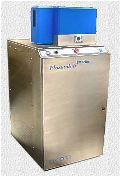
Fig. 3.5 The RIE system of Plasmalab 80 Plus: (a) an overall view (b) a schematic of reacting chamber with two parallel plates and a few hundred watts of RF electromagnetic field applied on it.
