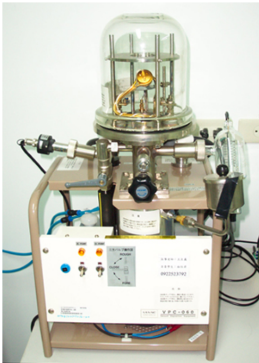
Fig. 3.6 An overall view of (a) the thermal evaporation machine (b) the e-beam evaporation machine.
