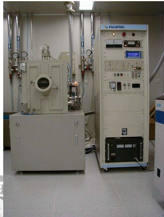
Fig. 3.6 An overall view of (a) the thermal evaporation machine (b) the e-beam evaporation machine.
