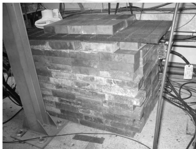
Figure 2.3: The computer inside the shielding is used for the beam spot monitor.
